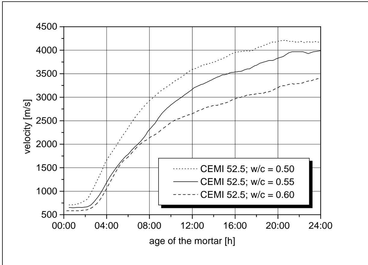
Fig. 5. Velocity of the US wave depending on the age of a mortar with CEM I 52.5 with variation of the water-cement-ratio.
