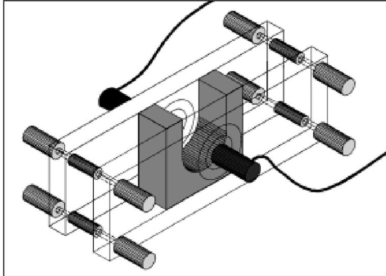
Fig. 2. Set-up for the mortar experiments showing the mould (rubber foam and PMMA walls) and the transducers.
