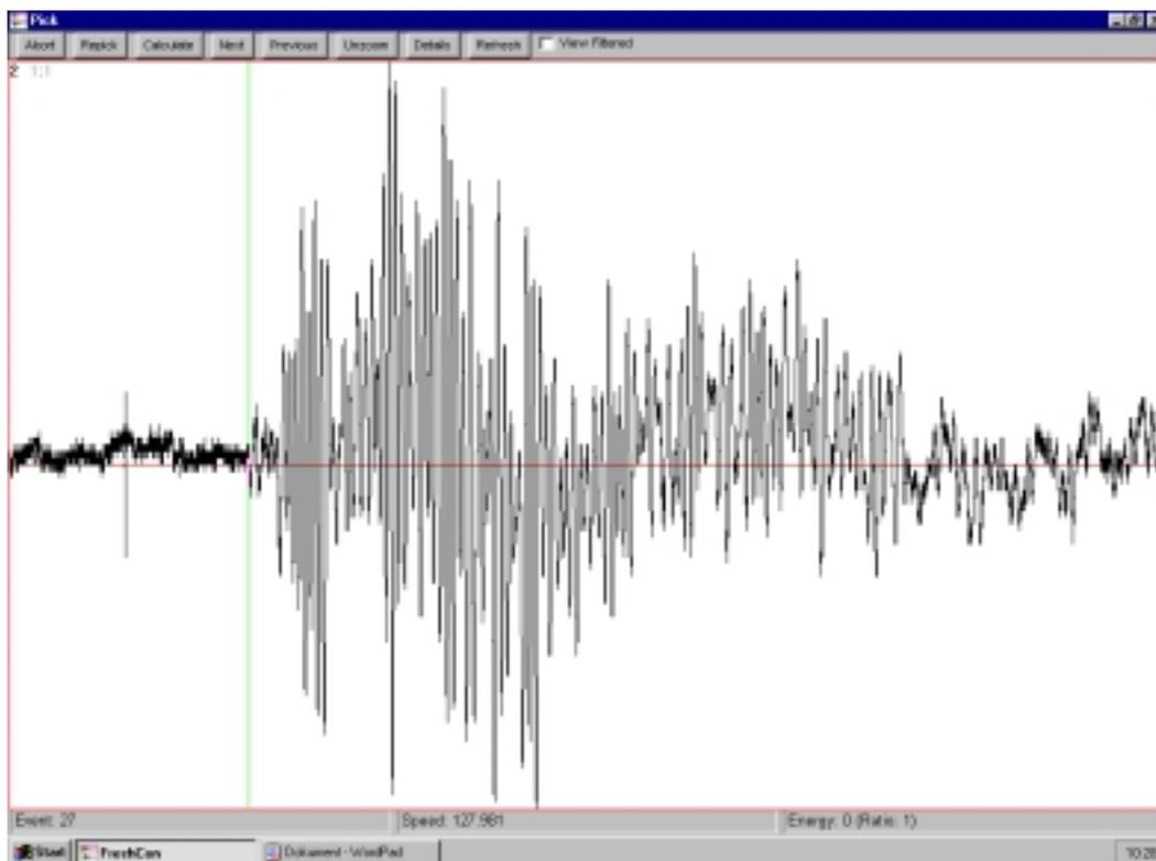
Fig. 3. Example of an unfiltered US signal in *FreshCon* using the semiautomatic picking mode.
