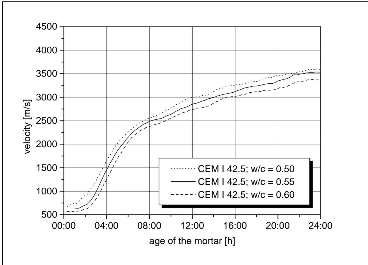
Fig. 4. Velocity of the US wave depending on the age of a mortar with CEM I 42.5 with variation of the water-cement ratio.
