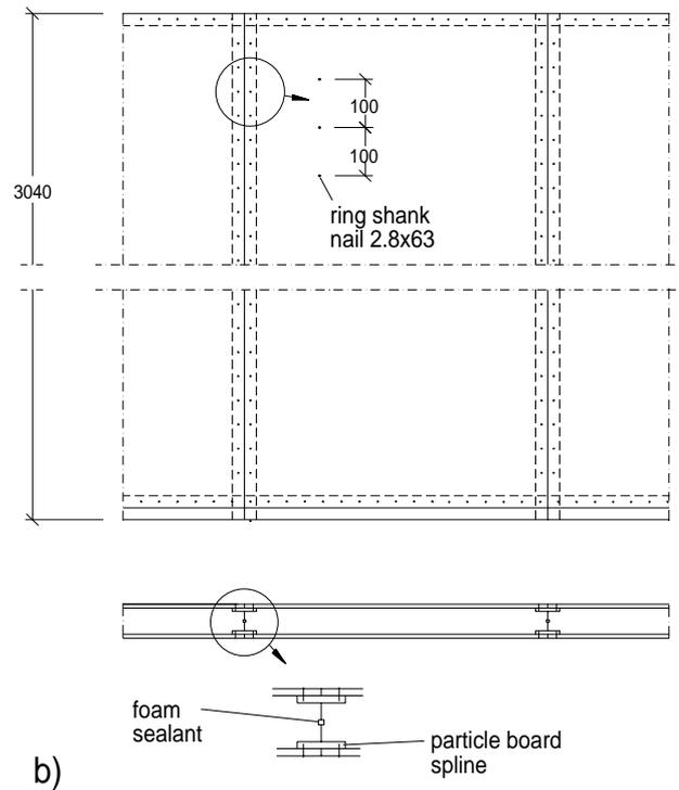
Fig. 1a, b. Built-up and dimensions of sandwich wall element and respective connection of adjacent elements acc. to building approval Z-9.1-315 (presently panel height is restricted to 2,75 m)
