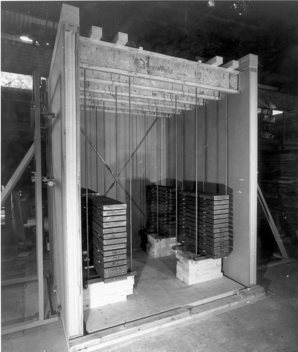
Fig. 6. *Photograph of the one-sided open test cabin after load application to the I-beams*
