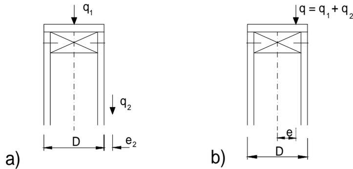
Fig. 2a, b. *Eccentricity definitions of partial and total vertical loads*
