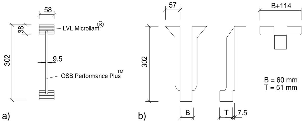
Fig. 3a, b. *Employed I-beams and hangers*
