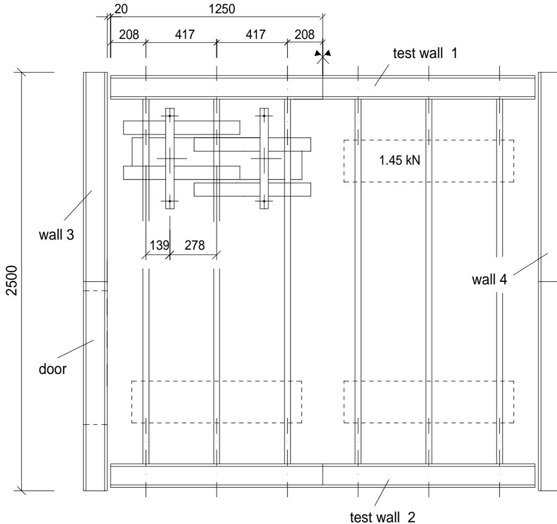
Fig. 5. Top view of the test cabin without roof element including load application at the top chords of the I-beams; the roof element is not indicated
