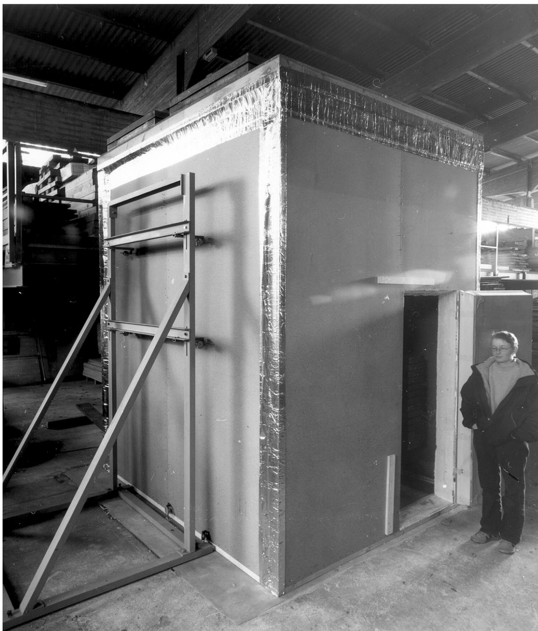
Fig. 8. *Photograph of the completely closed test cabin with diffusion tight sealing tapes along the edges*
