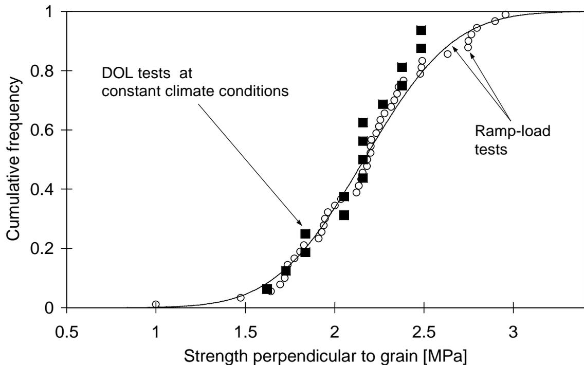
Fig. 5. Cumulative frequency of strength perpendicular to grain in DOL tests at constant climate conditions of 20°C / 65% RH; also given are the results and the fitted distribution of the ramp load tests.
