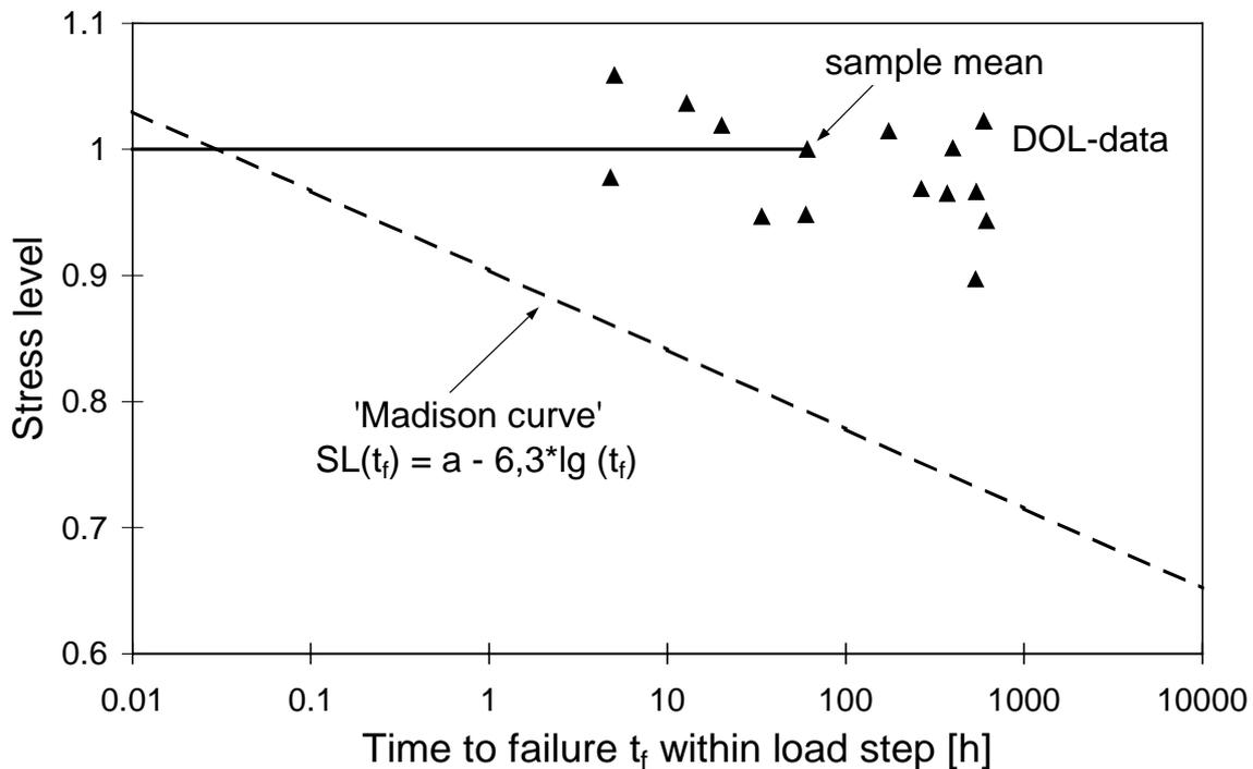
Fig. 6. Individual failure stress levels vs. time to failure within failure load steps; additionally given is the Madison curve, i.e. the expected DOL behaviour of wood
