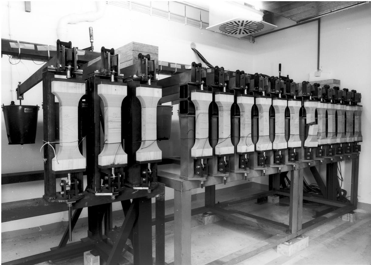
Fig. 3. *Photograph of realised long-term test set-up in the climate chamber*
