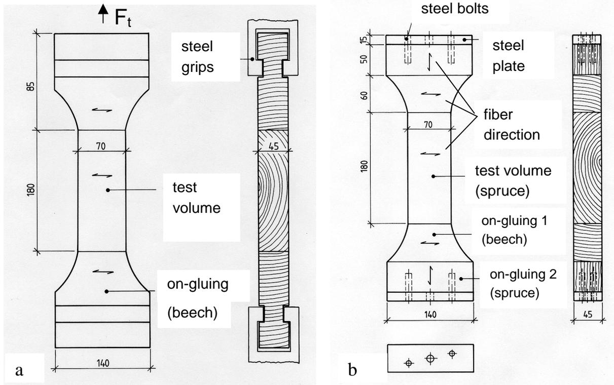
Fig. 1a, b. Sketches of developed specimen built ups slightly different for ramp load and long-term testing
