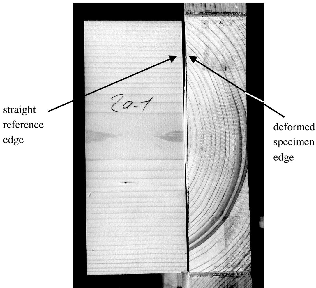
Fig. 7. Typical deformation shape of investigated spruce specimens long-term loaded in tension perpendicular to grain.
