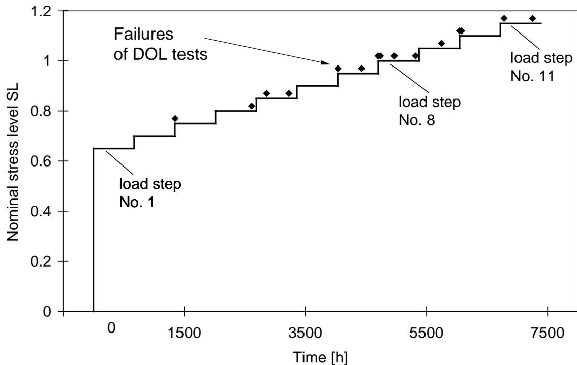
Fig. 4. Times to failure along load history with increased stepped nominal stress levels
