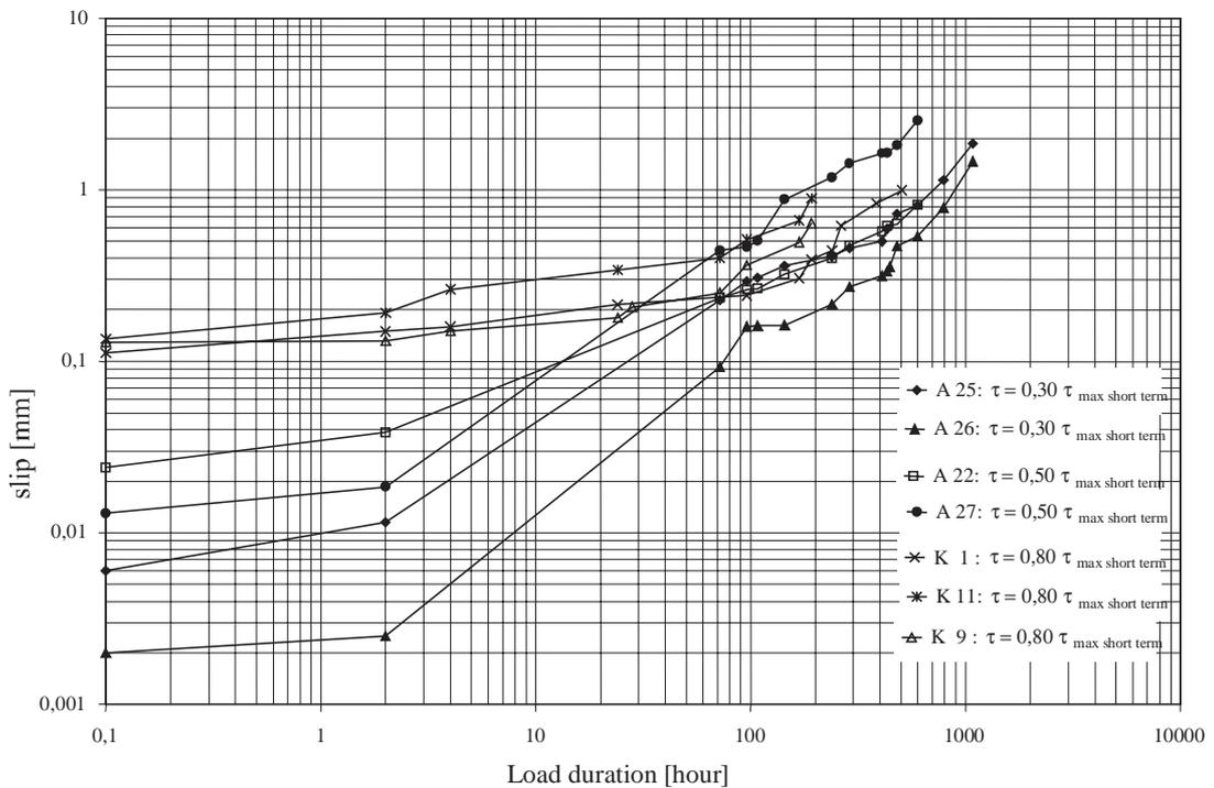
Fig. 6: Results of sustained pull-out tests with simultaneous thermal cycles.
