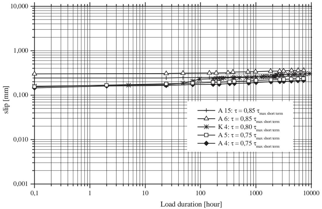
Fig. 5: Results of sustained pull-out tests in standard climate
