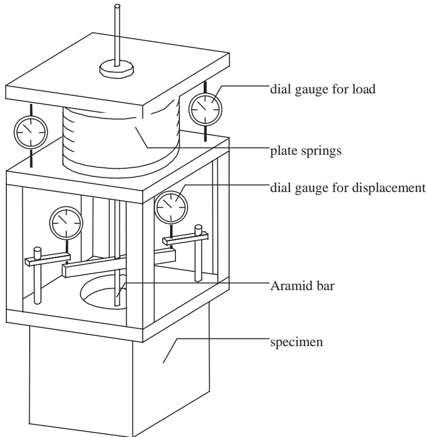
Fig. 3: *Long term loading equipment*
