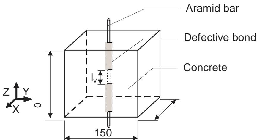
Fig. 1: *Cube with aramid bar used for pull-out tests*
