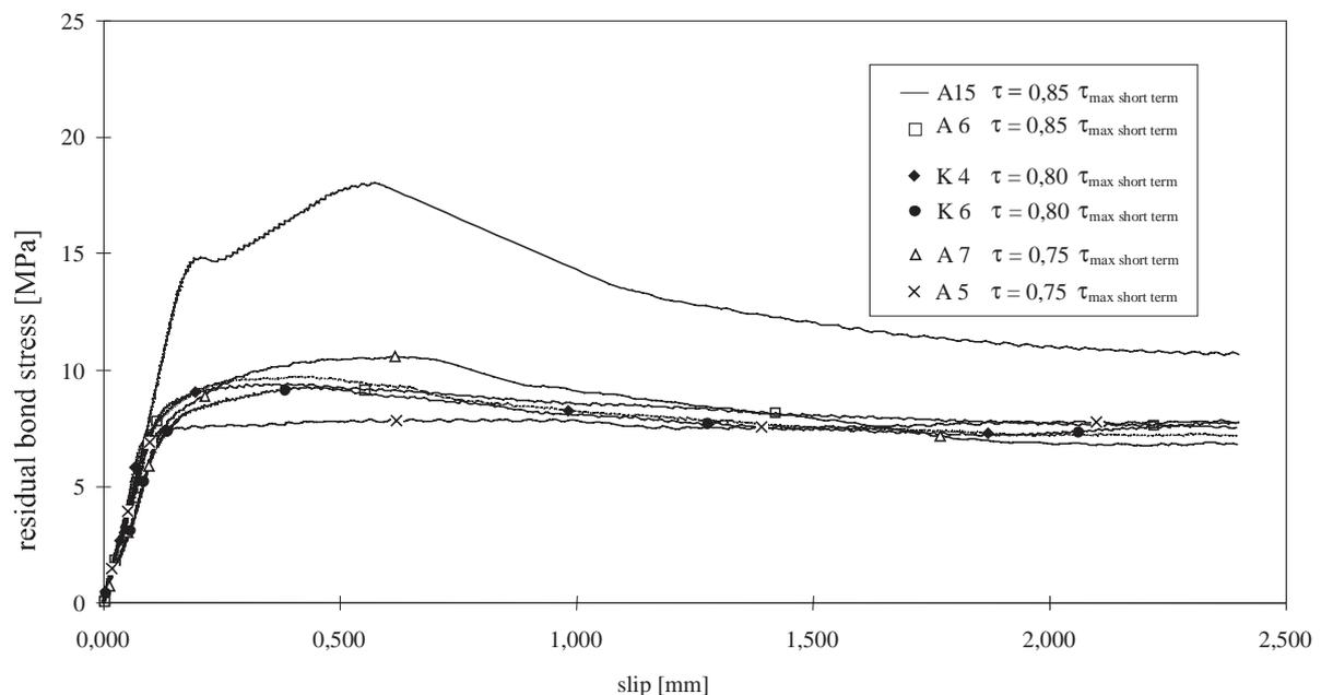
Fig. 7: *Residual bond stress vs. slip relation of specimens from standard climate*
