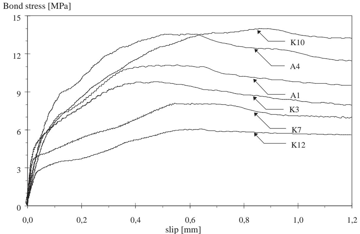
Fig. 4: *Bond stress vs. relative displacement as result of pull-out test*
