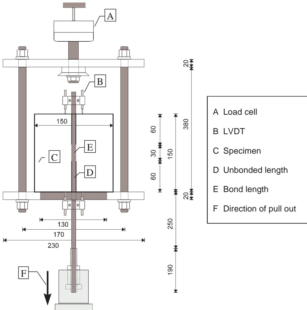
Fig. 2: Pull-out test equipment for short term test
