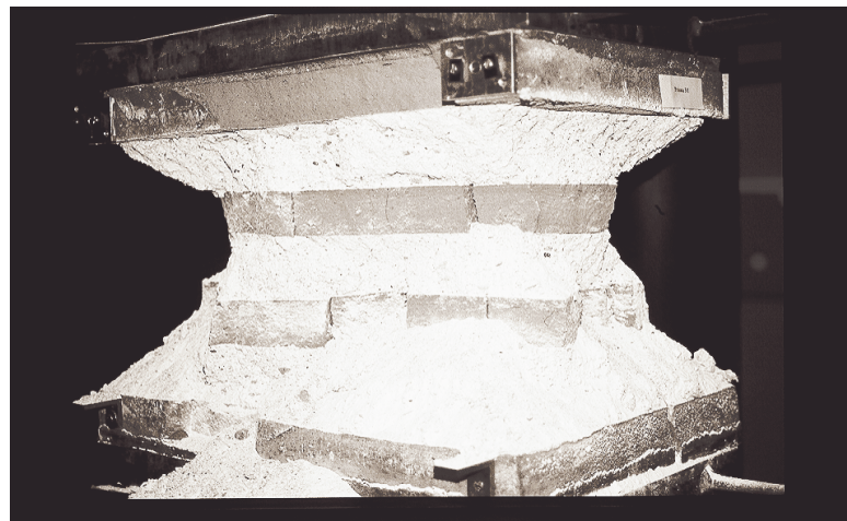
Fig. 4: Cracking and failure pattern of masonry prisms a) Prism 2/2 at \sigma = 2.5 MPa b) Prism 3/1 at \sigma = 2.9 MPa, prepeak c) Prism 3/1 at \sigma = 2.8 MPa, postpeak
