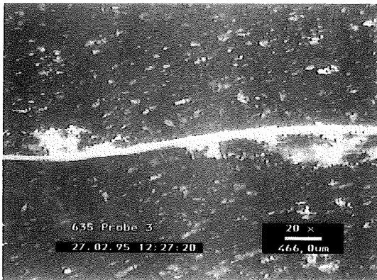
Fig.5 Bitumen top layer sheet of a flat roof sealing system with an unsaturated glass fibre fabric reinforcement.
