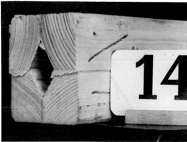
Figs. 6a, b: Typical shear fracture appearance of Cross-Beam viewed at end cross-section
