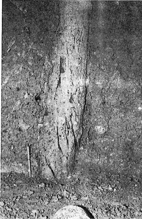
Fig. 5 Nail section near the shear plane after the test
