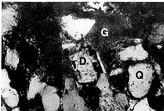
Fig.2: Fabric of the dolomitic variety 1 rich in Fe-hydroxides. Quartz light and dark grey (Q), dolomite (D) with brown Fe-hydroxide precipitated in the dissolved zone, glauconite (G) in greenish colours, pores dark. RGD 758-3, thin section, plane polarized light, magnification: small side of the picture \approx 1.5mm.
