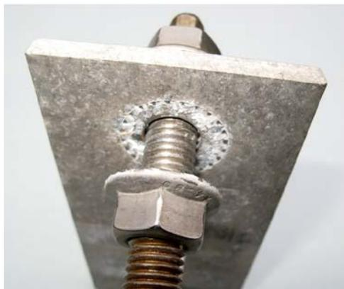
*Fig. 8: Aluminium flat steel with corrosion products in the contact area*
