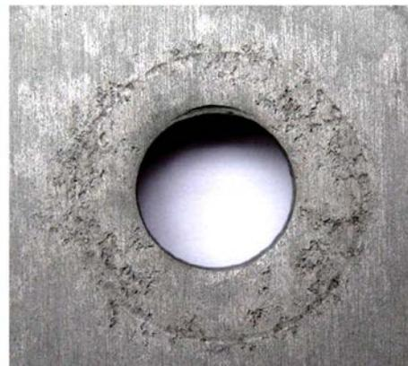
*Fig. 9: Flat steel after removal of the corrosion products from the contact area*
