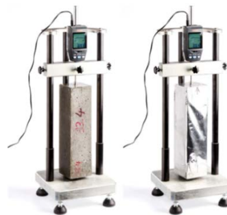
Fig. 2: Measuring instrument with dial gauge from Schleibinger - left with open prism - right packed with aluminium-laminated PE-foil
