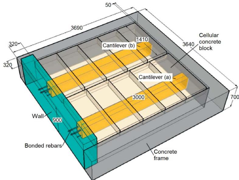
Fig. 2: Beam-wall connection configuration tested under fire [11] (All dimensions in mm)
