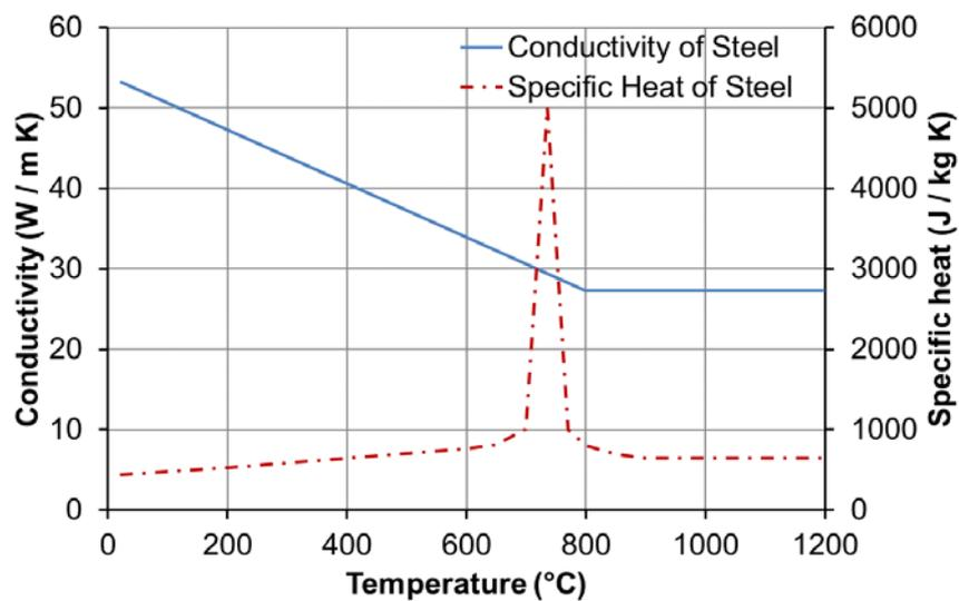
Fig. 7: Thermal properties of reinforcing steel as function of temperature
