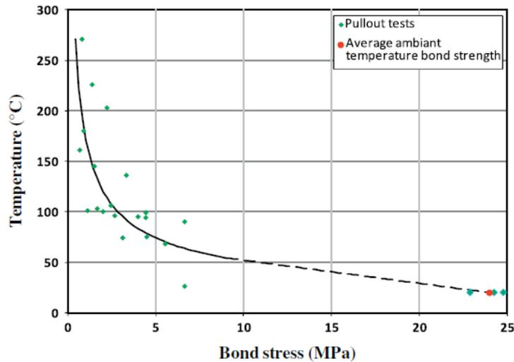
Fig. 4: Bond stress variation with temperature for the polymeric adhesive used by Pinoteau et al. [11]
