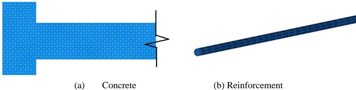
Fig. 5: Geometric discretisation of Cantilever beam-wall connection (FE mesh)
