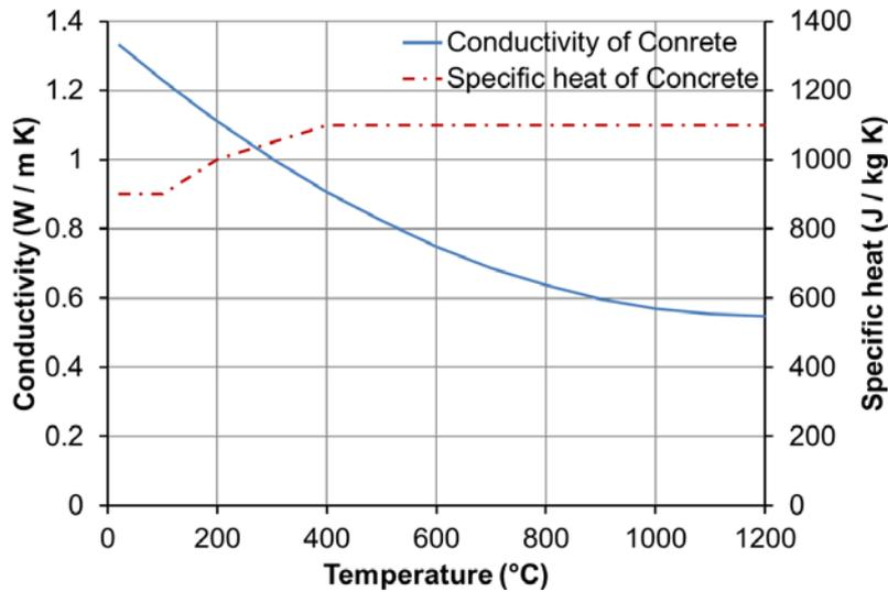
Fig. 6: Thermal properties of concrete as function of temperature
