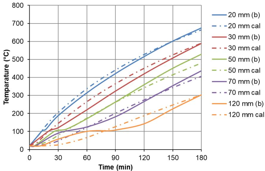
*Fig. 8: Temperature variation in the cantilever beam*
