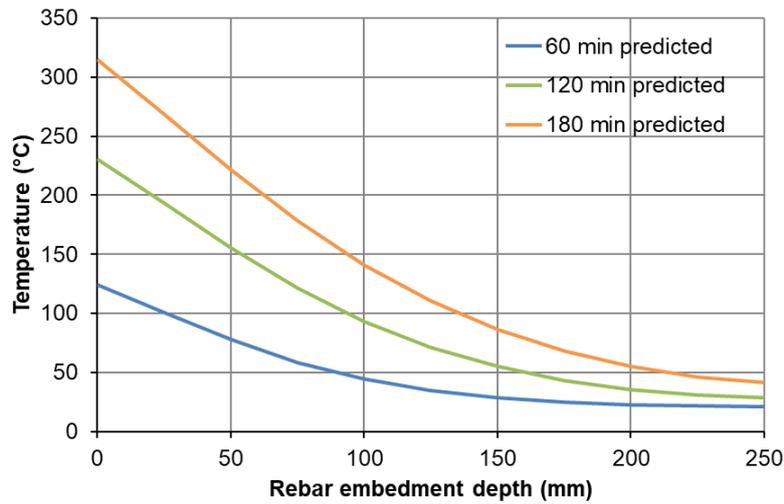
Fig. 9: Temperature variation along the embedment length of tension reinforcement in the cantilever beam
