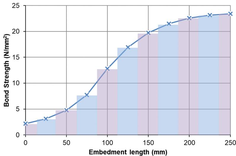
Fig. 1: Integration scheme for evaluating the pull-out capacity (Rectangular rule)
