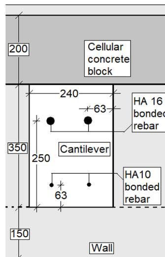
Fig. 3: Cantilever beam cross-sectional details (All dimensions in mm)
