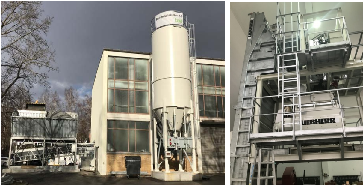
Fig. 3: Installation of a real-scale mobile concrete mixing plant type Liebherr DW 1,25 in the test hall Pfaffenwaldring 4d at the MPA University Stuttgart - pocket series silo with 4 rock grain chambers with externally mounted cement silo (left) and view of the mixing plant integrated into the hall (right) (source IWB)
