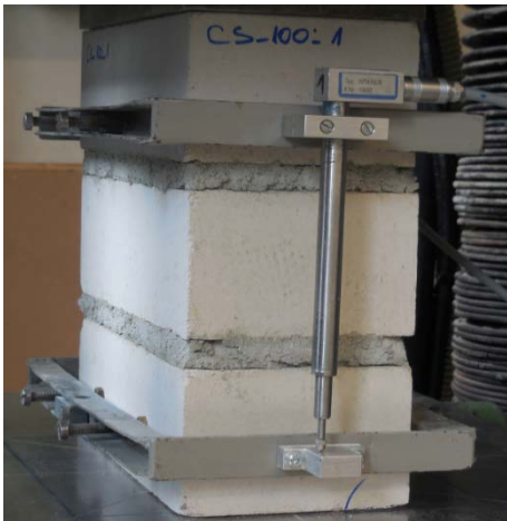
Fig. 2: Compression test on masonry prisms – test setup – a) Calcium silicate brick prism; b) Clay brick prism
