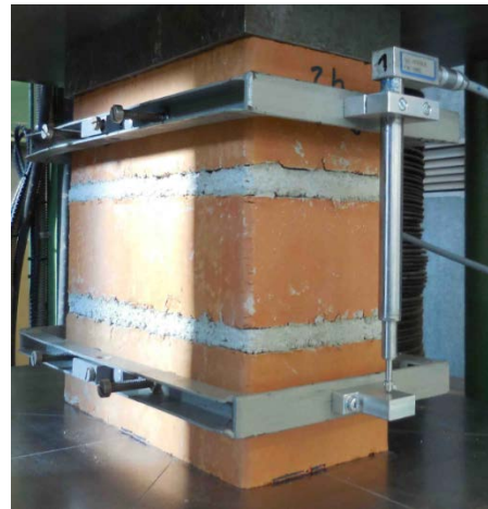
Fig. 2: Compression test on masonry prisms – test setup – a) Calcium silicate brick prism; b) Clay brick prism
