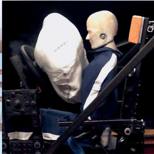
Dynamic sled for crash simulation
