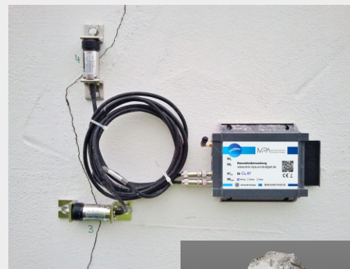
Instrumented crack monitoring with wireless sensor nodes
